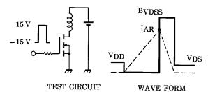
$$\begin{aligned} R_G &= 25~\Omega \\ V_{DD} &= 25~V,~L = 165~\mu H \end{aligned} \qquad E_{AS} &= \frac{1}{2} \cdot L \cdot I^2 \cdot \left( \frac{BVDSS}{BVDSS - VDD} \right) \end{aligned}$$
